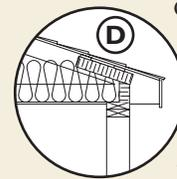
Older split-levels often have low-slope roof trusses that have very little height at the edge, leaving little room for insulation. The best choice here is blown-foam insulation, giving high R-values and good air sealing. Friction-fit high-density rigid board at the eaves will also give higher insulation values in this area but is more labour-intensive.
