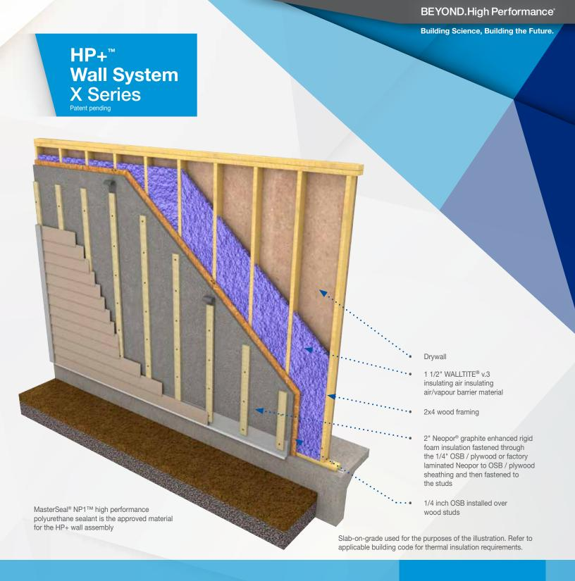
The HP+ Wall System X Series is a structural assembly that meets or exceeds codes with a minimum nominal insulation R-value of R-25 up to R-32 using 2 x 4 wood framing. The X Series offers exceptional strength against high winds and seismic movement.
